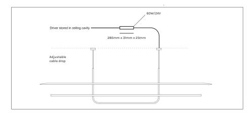
**INSTALLATION** Driver stored in ceiling cavity
